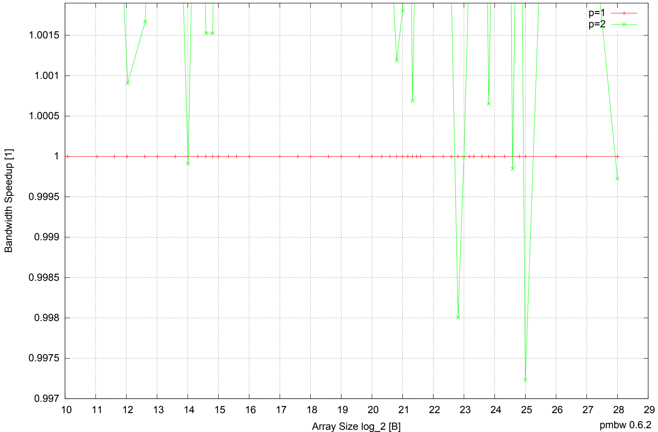
Raspberry Pi Model B: ARM1176JZF-S 512MB - Speedup of Parallel Memory Bandwidth (enlarged) - ScanWrite32PtrUnrollLoop
