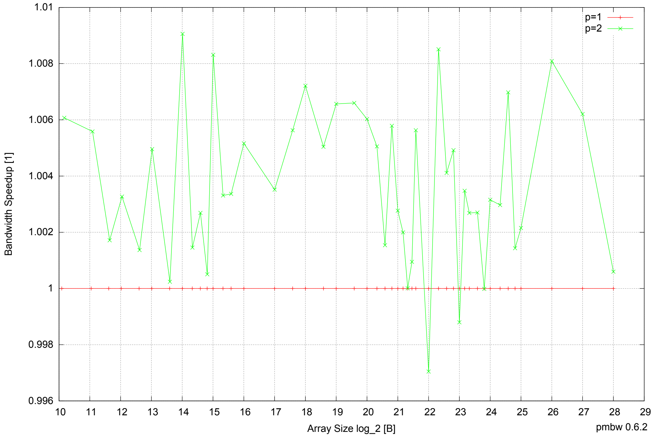
Raspberry Pi Model B: ARM1176JZF-S 512MB - Speedup of Parallel Memory Bandwidth - ScanWrite32PtrMultiLoop
