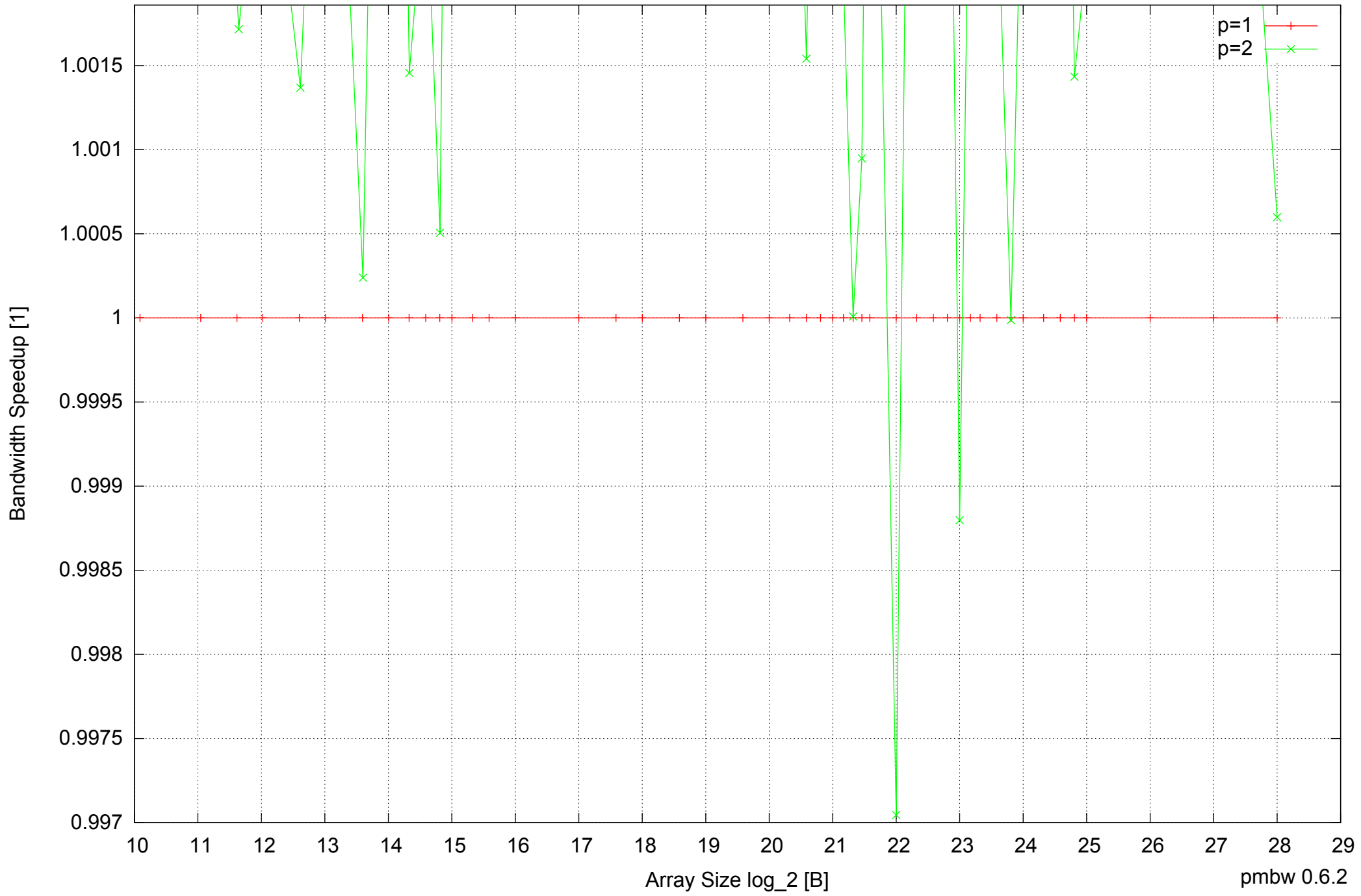
Raspberry Pi Model B: ARM1176JZF-S 512MB - Speedup of Parallel Memory Bandwidth (enlarged) - ScanWrite32PtrMultiLoop
