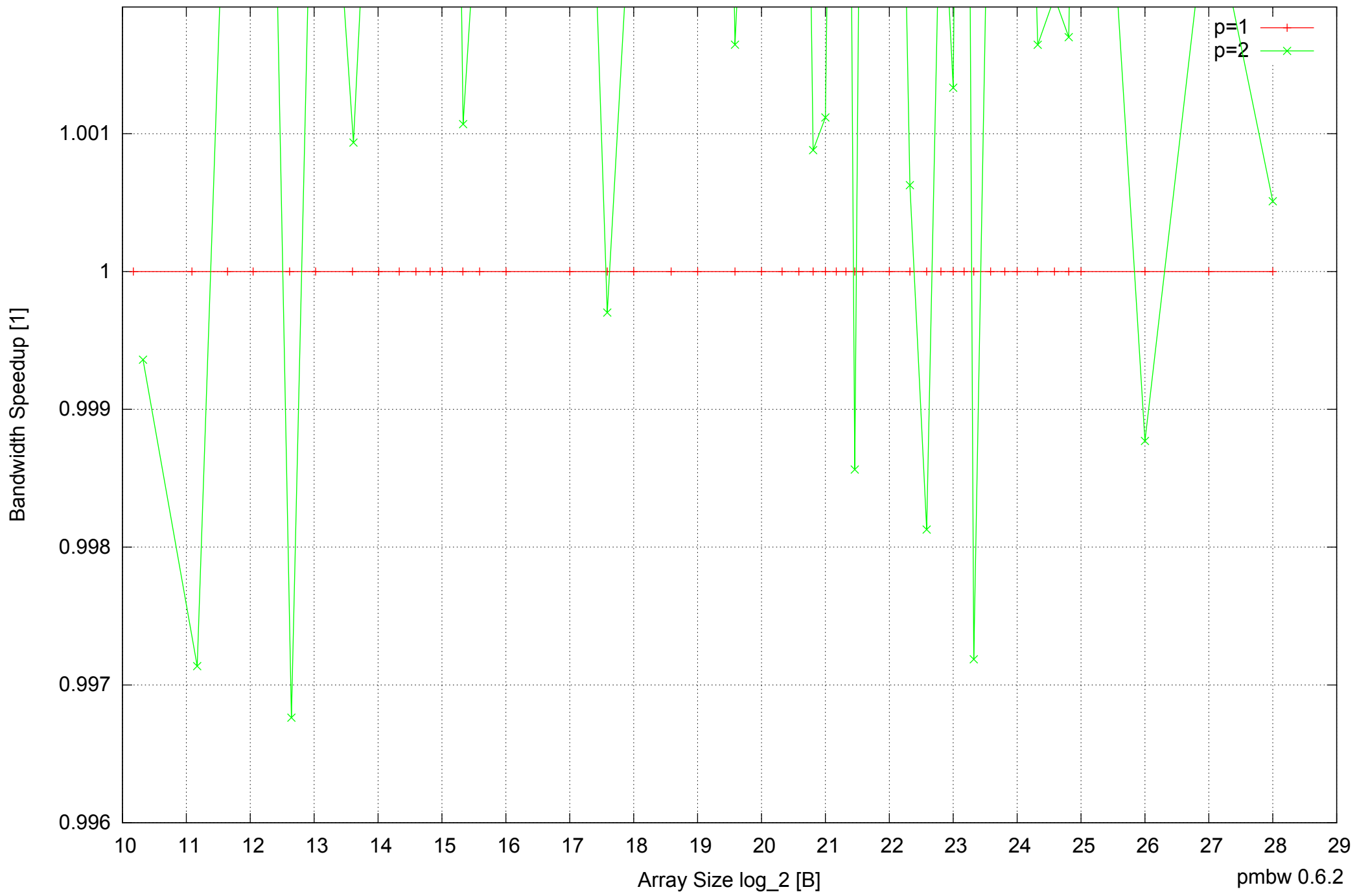
Raspberry Pi Model B: ARM1176JZF-S 512MB - Speedup of Parallel Memory Bandwidth (enlarged) - ScanWrite64PtrUnrollLoop
