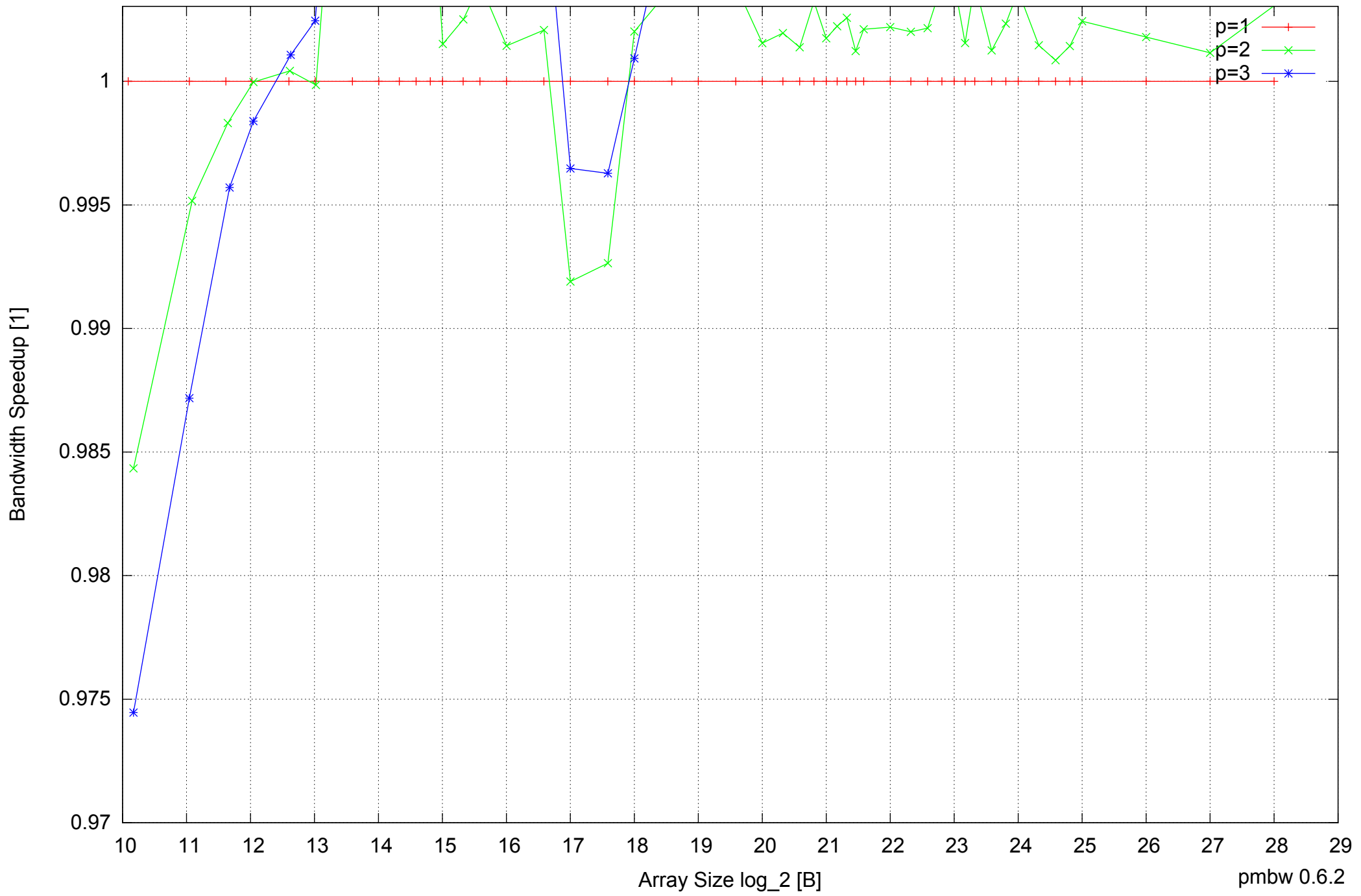
BeagleBone Black: AM335x 1GHz ARM Cortex-A8 512MB - Speedup of Parallel Memory Bandwidth (enlarged) - ScanWrite32PtrSimpleLoop
